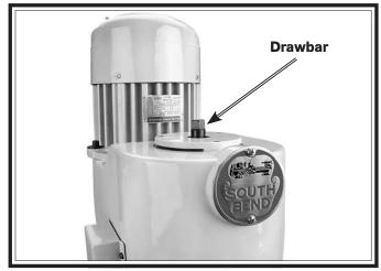
Figure 44. Drawbar loaded into the spindle.
